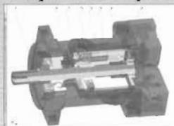
*Interaction simulation of axial-piston hydromachines running gear details using MSC.AFEA (part 1)*
