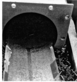
Fig. 3: Shaftless screw, U-shaped polyethylene wear-resistant liner (Source: DIM GmbH, ImRo Bückeburg)
